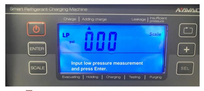
Press the button to begin the process. The Charging Station will enter an Evacuation and Holding test for **INTERNAL** piping only, to remove possible contaminants from the unit before adding the charge.
