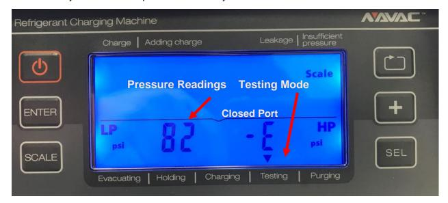
7. You can skip over Testing Mode by pressing the "Sel" button and go to Purging.
