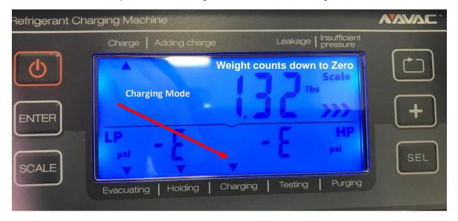
6. Once the Charging is finished, the unit will beep 3X and advance to testing mode. Here you can see the pressures of the system.
